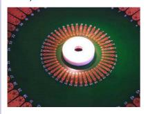
Capitalizing on its solid experience in parametric testing, Synergie CAD Group has expanded its line and is now offering probe cards compatible with Agilent 4060 and 4070 series. Technics used to manufacture these parametric probe cards are similar to the ones used for Keithley compatible series, but different boards are used. We manufacture probe cards using all technologies available at Synergie CAD.
